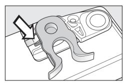
■ Using a screwdriver, remove spring clamp <sup>③</sup> from underneath the door and fit it on the opposite side.
